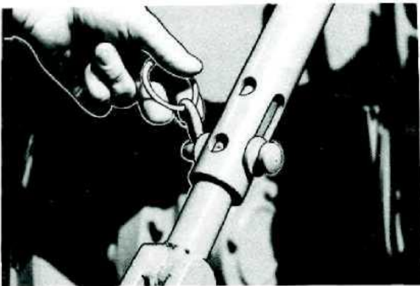
Fig. P.6 — Lift Arm Pins in Slotted Holes.
