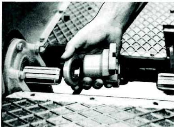
Fig. H.5 — Removing Main Coupling shaft yoke.
