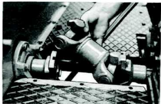
Fig. H.4 — Removing Main Coupling shaft
