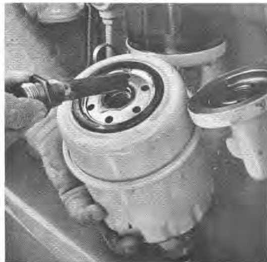
Fig. B11 — Fitting Standpipe to New Engine Oil Filter
