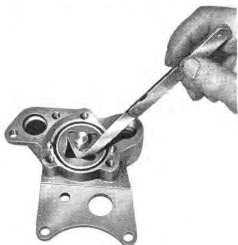
Fig. B58 — Checking Inner and Outer Rotor Clearance
