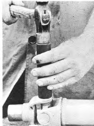
Fig. H6 — Drifting the Bearing
