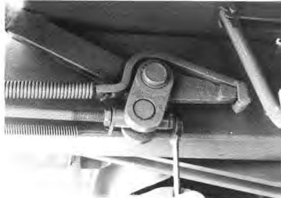
Fig. F2 — Clutch Pedal Adjustment
