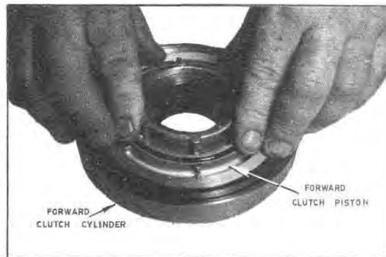
Fig. G61 — Install the Forward Clutch Piston
