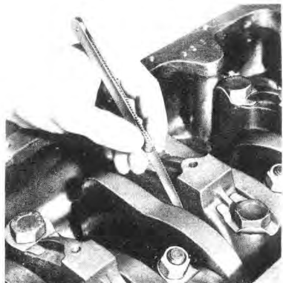
Fig. B33 — Checking the Crankshaft End Float
