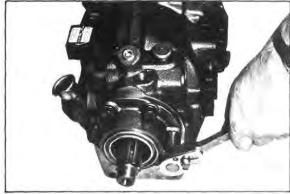
Fig. G90 — Tightening the Adaptor Bolts
