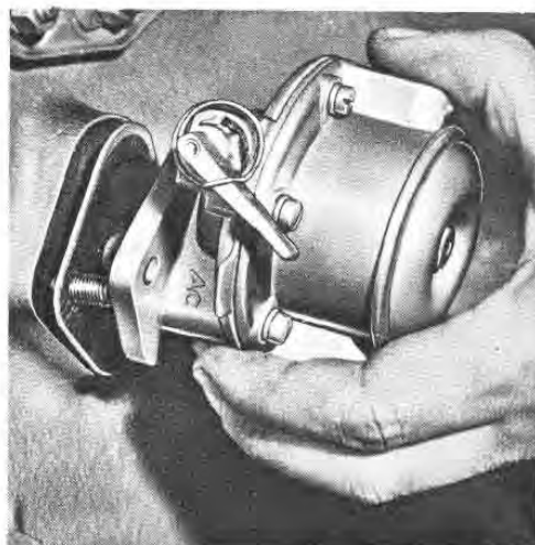
Fig. B43 — Removing the Fuel Lift Pump
