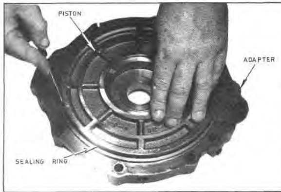
Fig. G81 — Assembling the Reverse Clutch Piston
