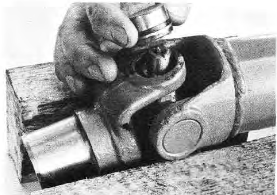
Fig. H8 — Removing the Opposite Bearing
