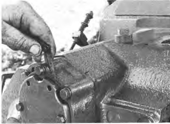
Fig. G11 — Measuring Mainshaft Retainer Clearance
