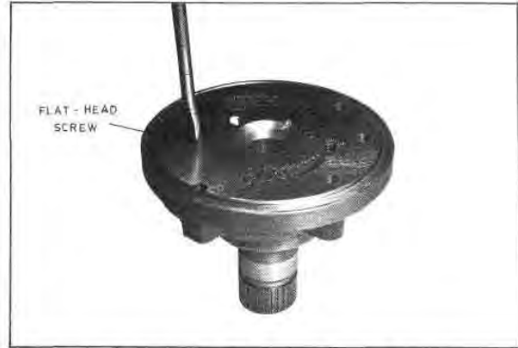
Fig. G17 — Removing the Pump Retainer Screw
