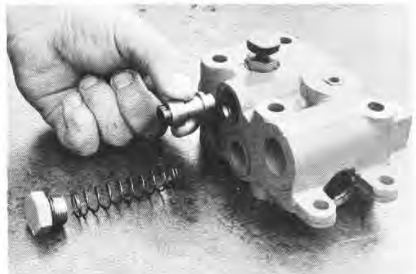
Fig. 013 — Correct Relief Valve Installation
