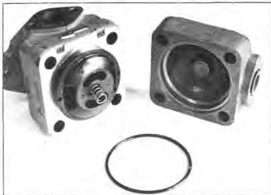
Fig. O4— Pump Cover Removed
