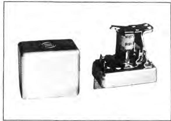
Fig. E11 — The Voltage Regulator (cover removed)
