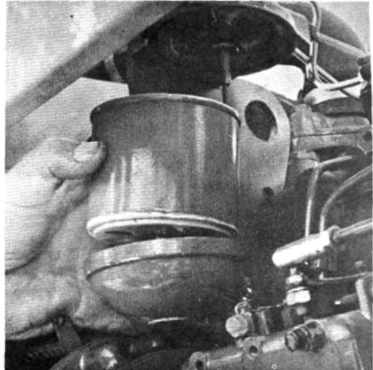
Fig. D7 — Removing the Final Fuel Filter
