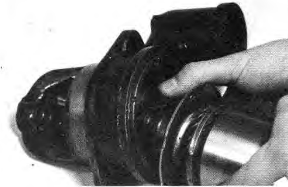
Fig. E16 — Pull the Drive End Plate Forward
