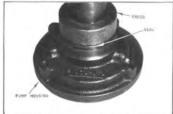
Fig. G83 — Assembling the Oil Seal
