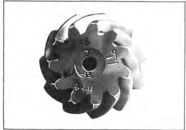
Fig. K5 — Pinion Head Core Plug Marking
