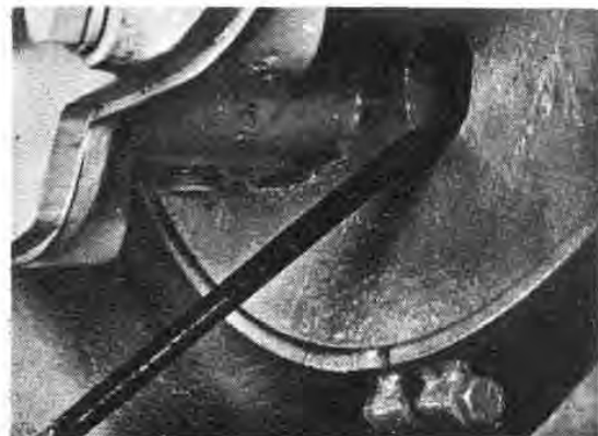
Fig. N3 — Adjusting Brake Shoes
