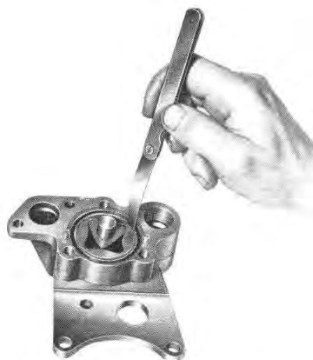
Fig. B59 — Checking Outer Rotor to Body Clearance
