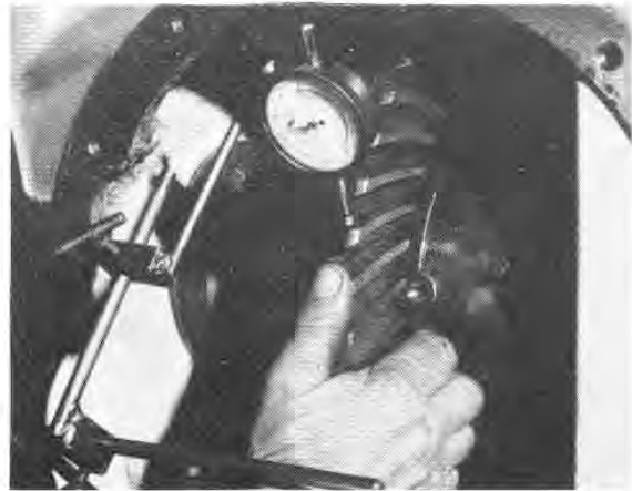
Fig. K9 — Checking Crownwheel Backlash
