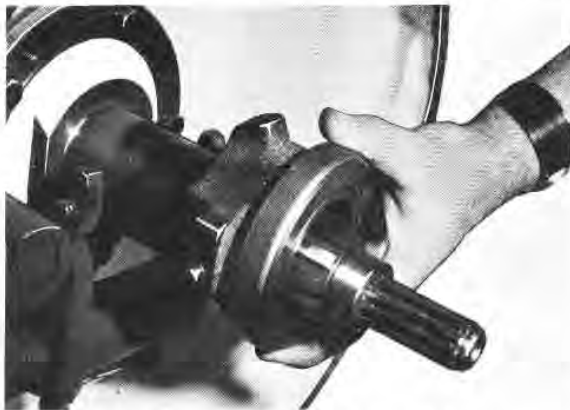
Fig. F9 — Throw-out Bearing and Carrier Removal
