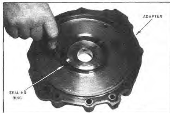
Fig. G80 — Assembling the Adaptor Hub Sealing Ring
