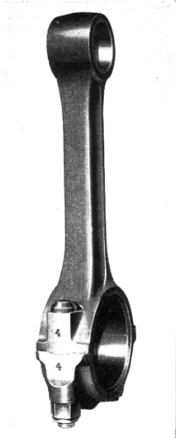
Fig. B26 — Connecting Rod and Cap Numbering
