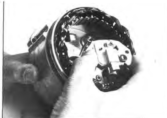
Fig. E9 — Alternator Brush Holder Removal
