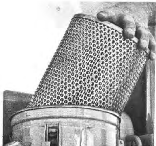
Fig. B6 — Remove Dry Air Cleaner Element
