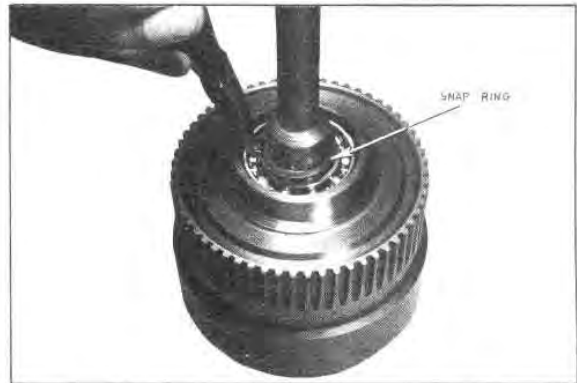
Fig. G29 — The Drive Gear Bearing Snap Ring
