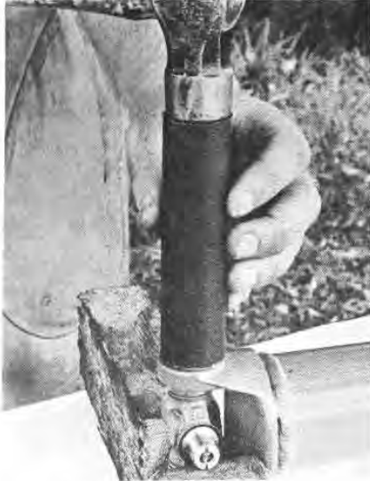
Fig. H9 - Drifting Second Pair of Bearings
