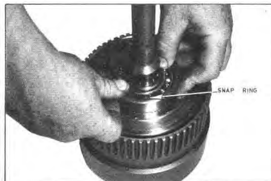
Fig. G71 — Installing the Clutch Cylinder Snap Ring
