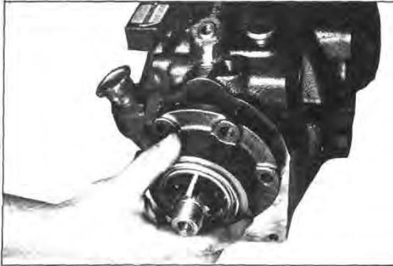
Fig. G89 — Positioning the Rear Adaptor
