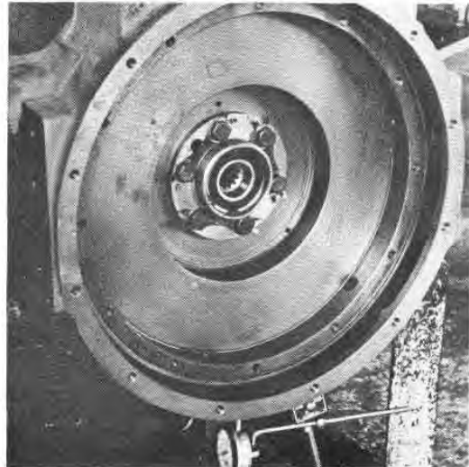
Fig. B48 — Alignment of Flywheel Periphery
