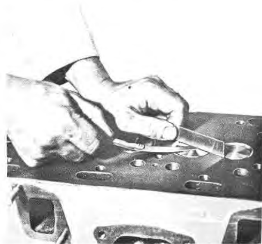
Fig. B15 — Checking Valve Depths
