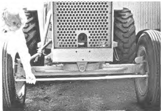
Fig. A29 — Checking Wheel Alignment
