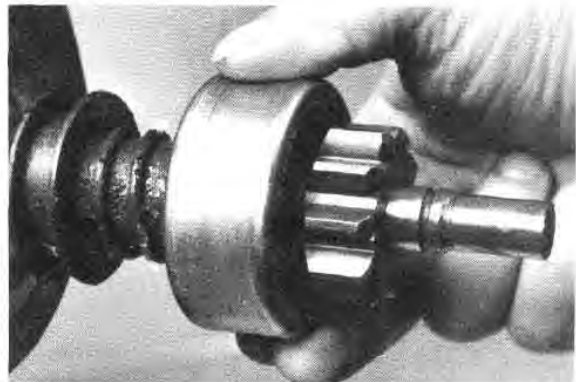
Fig. E19 — Sliding the Drive Assembly off the Armature Shaft
