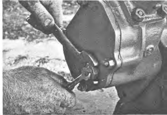
Fig. A13 — Rocker Shaft Screw Adjustment
