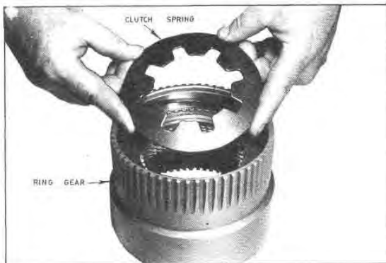
Fig. G58 — Install the Clutch Spring
