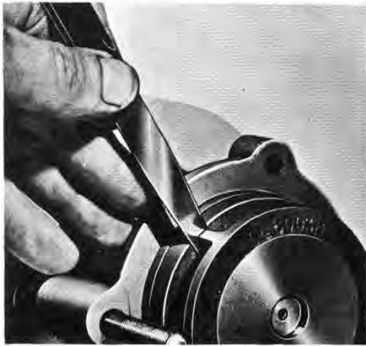
Fig. C5 — Checking the Impellor to Water Pump Body Clearance
