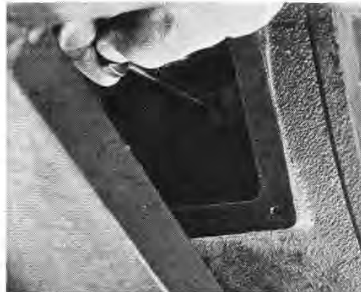
Fig. F15 — Draining the Converter
